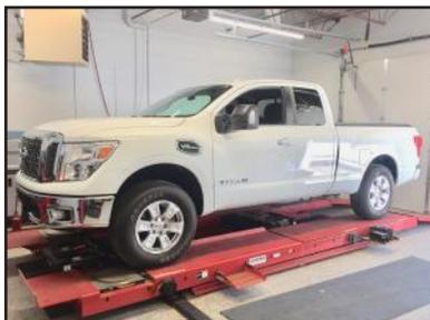
**STEP 2:** On a flat, level surface, MEASURE preinstallation ride height, FRONT & REAR, and write down measurements.
