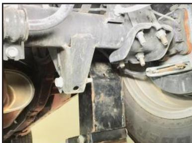
**STEP 4:** Loosen and remove OEM ubolts, nuts and plate.
