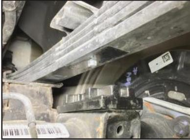
**STEP 8:** Install lift block, 1.5" height shown.
