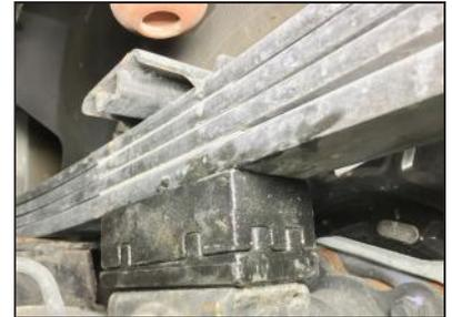
**STEP 11:** Install new Ubolts provided with the kit. Install spring bracket and install washers and nuts.
