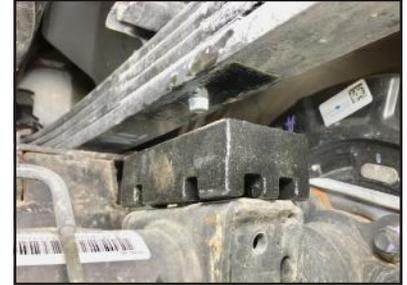
**STEP 9:** Install lift block, 2.0" height shown.
